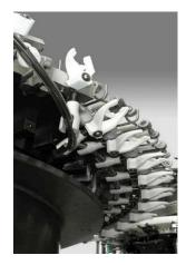
In the past, fillers were mainly "mechanical" fillers where individual steps of the filling process were mechanically initiated through cams/levers, pushbuttons and rollers. Today, electro-pneumatically controlled solenoids are employed on the filling valves. This guarantees a high degree of accuracy, reduces the amount of wear parts and facilitates product change overs through parameter setting on a filler touch screen.
