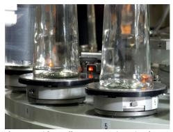
Photo 8: Side-wall Lug Detection via Photo-Electronic Sensor
