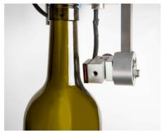
Photo 7: Embossing Detection via sensor (Peregrine Mobile Bottling)
