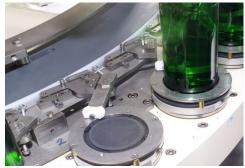
Photo 4: Mechanical Orientation for Side-wall Lug on Labeler Bottle Table
